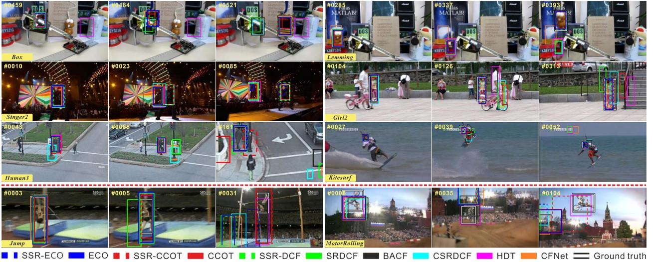
Fig. 9. Visualization results of SSR-ECO, ECO, SSR-CCOT, CCOT, SSR-DCF, SRDCF, and other four CF trackers. The first six sequences show the advantages of SSR-based CF trackers in handling occlusion and background clutter. The last two cases show the limitation of SSR-based CF trackers in handling fast motion with huge deformation.
