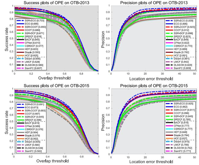
Fig. 6. Comparison results on OTB-2013 [26] and OTB-2015 [27]. The legend of each tracker shows the AUC score of success plots and precision at 20 pixels of precision plots.
