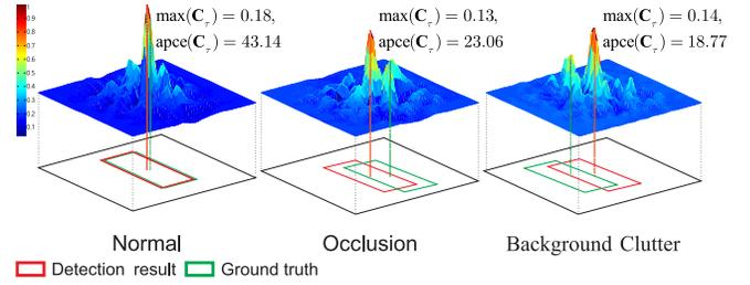
Fig. 4. Three examples of response maps, i.e.,  $\mathbf{C}_\tau$ , under situations of normal, occlusion and background clutter, respectively. The red rectangles show the detect results according to maximum of  $\mathbf{C}_\tau$ . The green rectangles show the ground truth.
